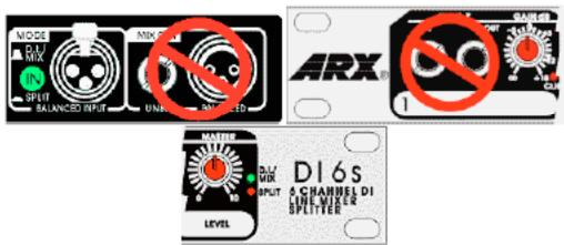
Please Note: In Splitter mode NO signal will be present on the MIX Output, and inputs via the Jack inputs SHOULD NOT be plugged in.
