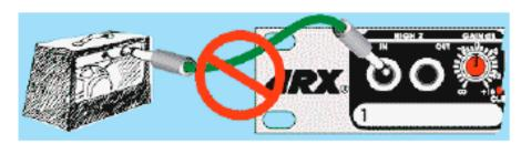
The DI6s is not designed to directly accept Amplifier output/speaker level signals. However, if you must capture that distinctive guitar amp sound without miking the speakers, or you've simply run out of microphones (don't laugh, it happens) then you can install the following circuit into a suitable ABS or discast Box.In the diagram below it is the Black Box!
