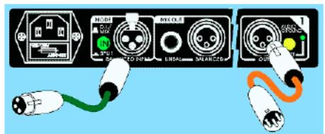
The signal from the Balanced XLR input on the rear panel is controlled by the Master control which varies the amount of input signal. This signal is then fed to each of the 6 individual channel balanced output XLR connectors where the individual output levels can be set.
